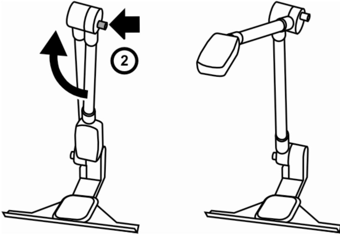
*Figure 3: Press and hold release button (2) to raise camera arm*
